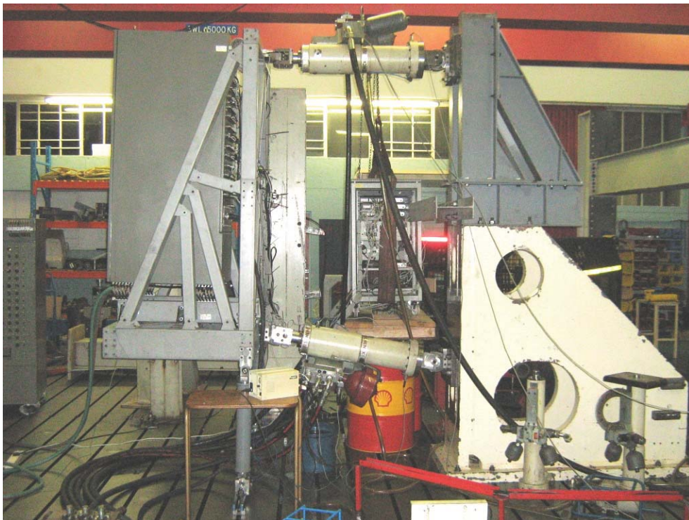
Figure 1.3: Two-axis shock and vibration test on defence industry electronics.
