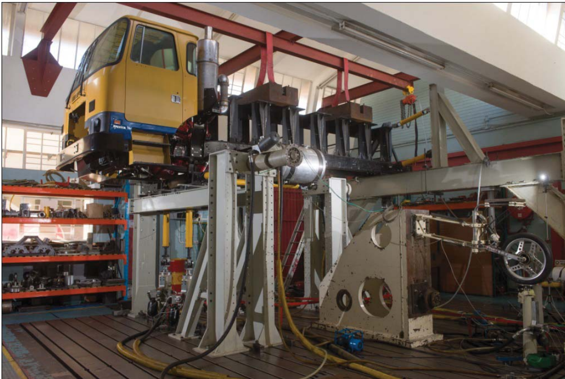
Figure 1.1: Six-axis durability test on Class 8 truck.
