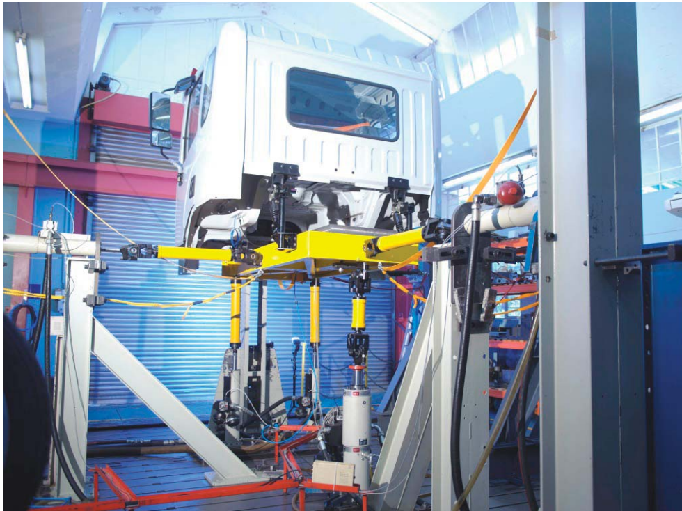
Figure 1.2: Five-axis durability test on a Class 7 truck cab.
