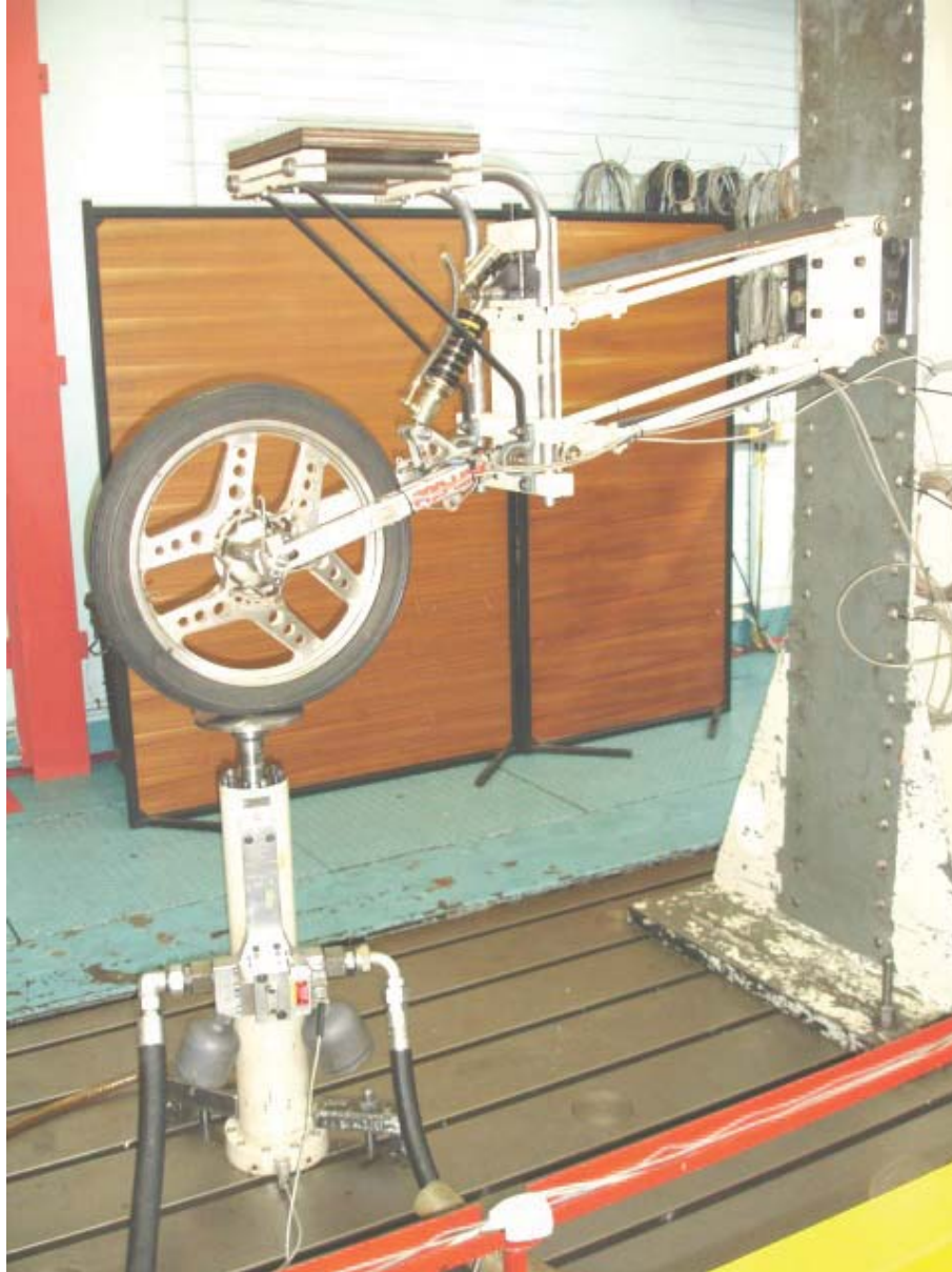
Figure 4.7: Quarter vehicle road simulator test rig.
