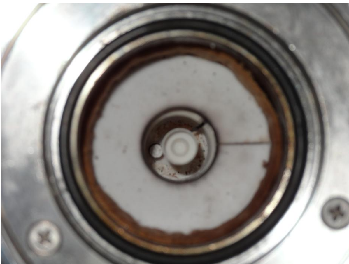
Figure 30: Top down view of the furnace with sample pan in place.
