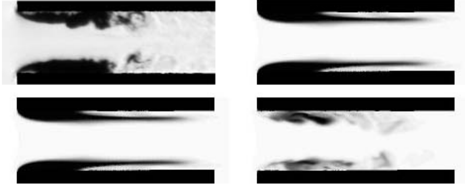
Figure 13: I-channel: (Upper left) Transmitted light, cf. Fig. 3; (Upper right) computed density field (white: liquid) of URANS for pressure difference of 300 bar – 120 bar, (Lower left) SAS and (Lower right) WALE-LES
