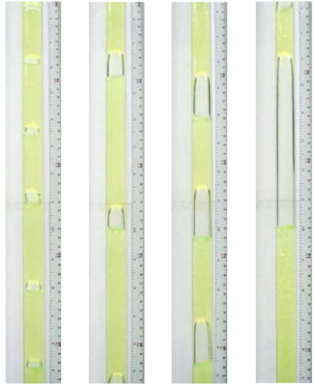
Figure 3 Flow regimes during the flow cycles in the riser
