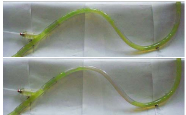
Figure 4 Gas accumulation and flushing at the bend.
