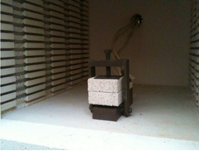
Figure 3. Specimen inside the high temperature oven.
