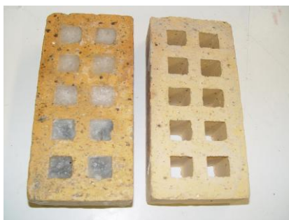
Figure 6: Picture of tested bricks. Right: hollow brick. Left: brick filled with the PCM – polymer composite. Experimental set-up and procedure
