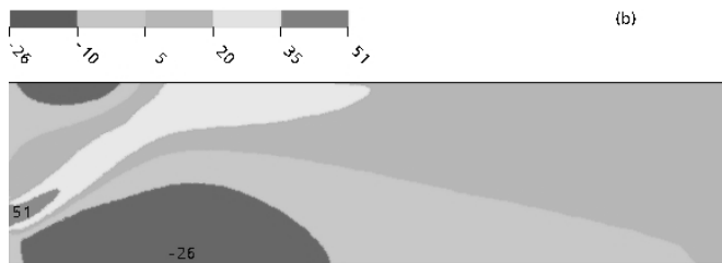
Figure 6 Predictions of axial velocity field for reactor diameter 75 mm. The results have been obtained for a premixed NG/NITROX system with equivalence ratio 3.1, pressure 6 bar and initial temperature 673 K. The numbers which appear in the pictures denote the maximum value (50 or 51 m/s) or the minimum value (-23 or -26 m/s) of the axial velocity. Values in between follow the grey scale shown in the legend.
