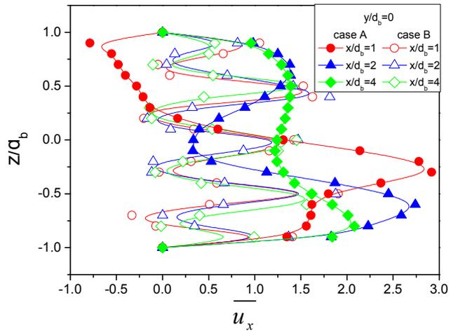
**Figure 6** Normalized time-averaged velocity distributions in different  $x$  planes at  $y/d_b = 0$
