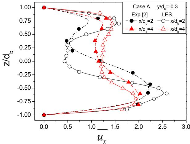
**Figure 2** Normalized mean velocity distributions in different  $x$  planes at  $y/d_b = -0.3$
