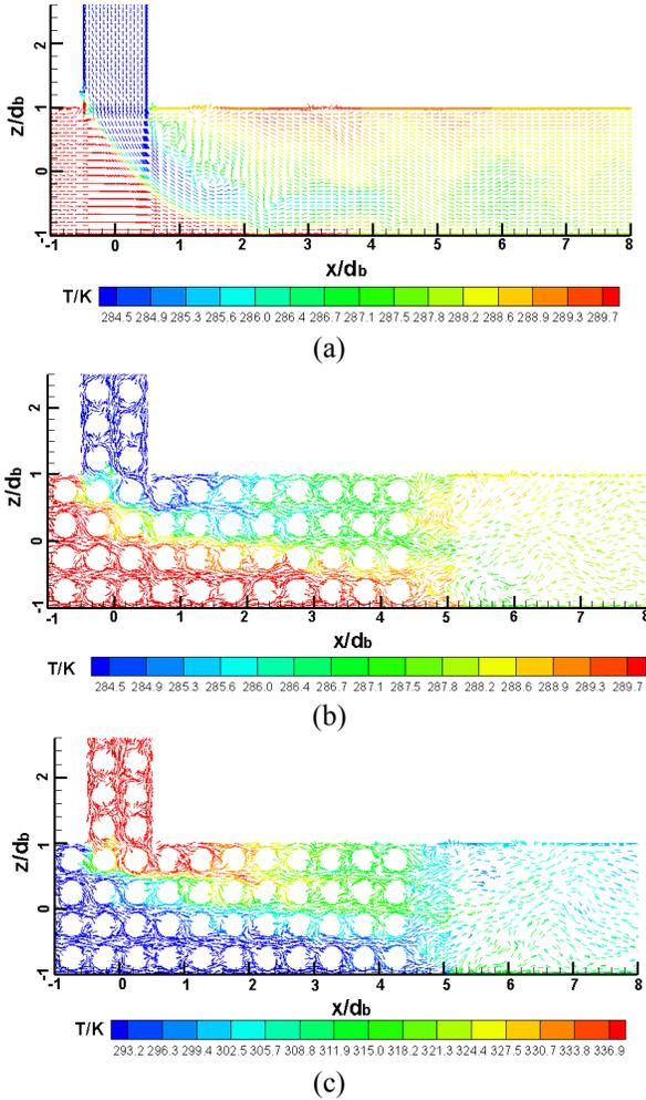
**Figure 4** Combined temperature and velocity vector distributions in the  $y/d_b=0$  plane at 13s. (a) Case A without porous medium,  $Ri = -0.093$ ; (b) Case B with porous medium  $Ri = -0.093$ ; (c) Case C with porous medium,  $Ri = 0.517$ .
