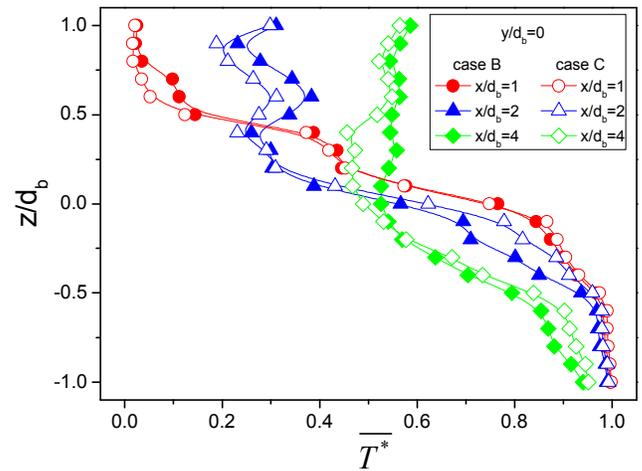
Figure 9 Normalized temperature distributions in different x planes at  $y/d_b = 0$
