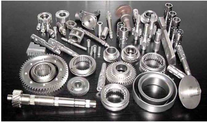
Figure 1. Different steel elements after high-pressure gas quenching.
