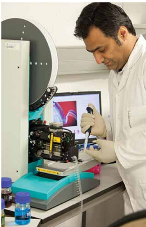
A robot can be employed to optimise the use of purified protein during crystallisation. A robot can dispense much smaller amounts of protein than a human can do by hand.
