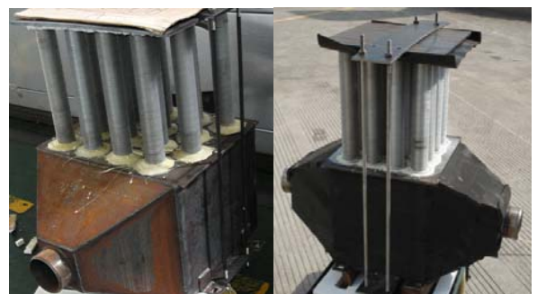
a. In-line arrangement b. In staggered arrangement Fig. 4 Small size samples in line & staggered arrangement
