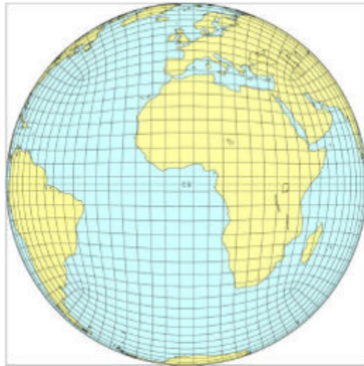
Figure 2.2.1: Illustration of the cube projected onto the globe at 200 km resolution (McGregor, 2006)
