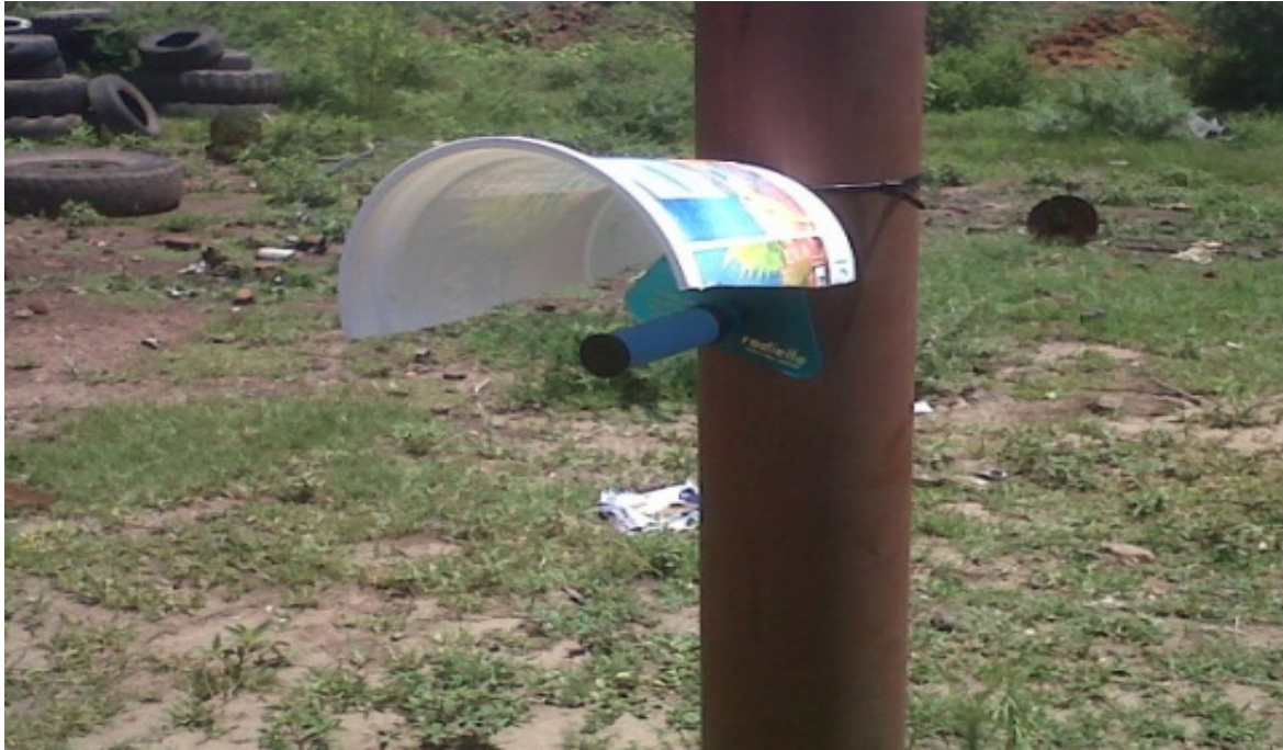
Figure 3-17: Radiello passive sampler installed on a supporting triangle and a plastic shield
