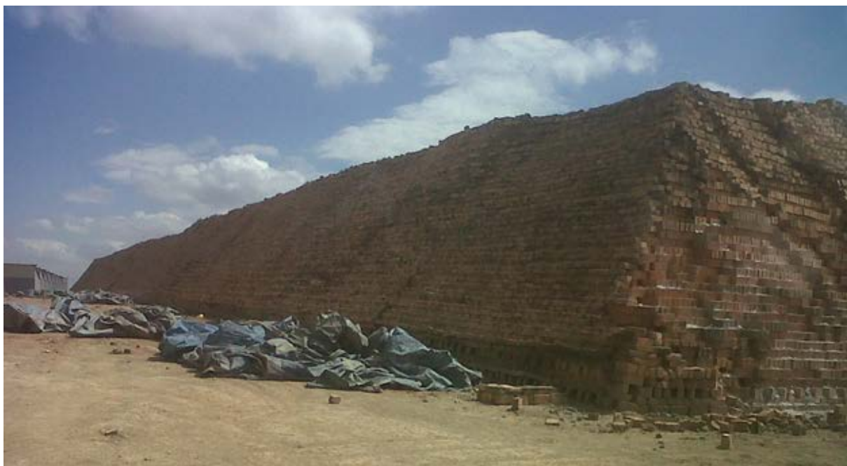
Figure 2-3: Red brick kiln at Bert’s Bricks, Potchefstroom firing over seven million bricks in less than 3 weeks
