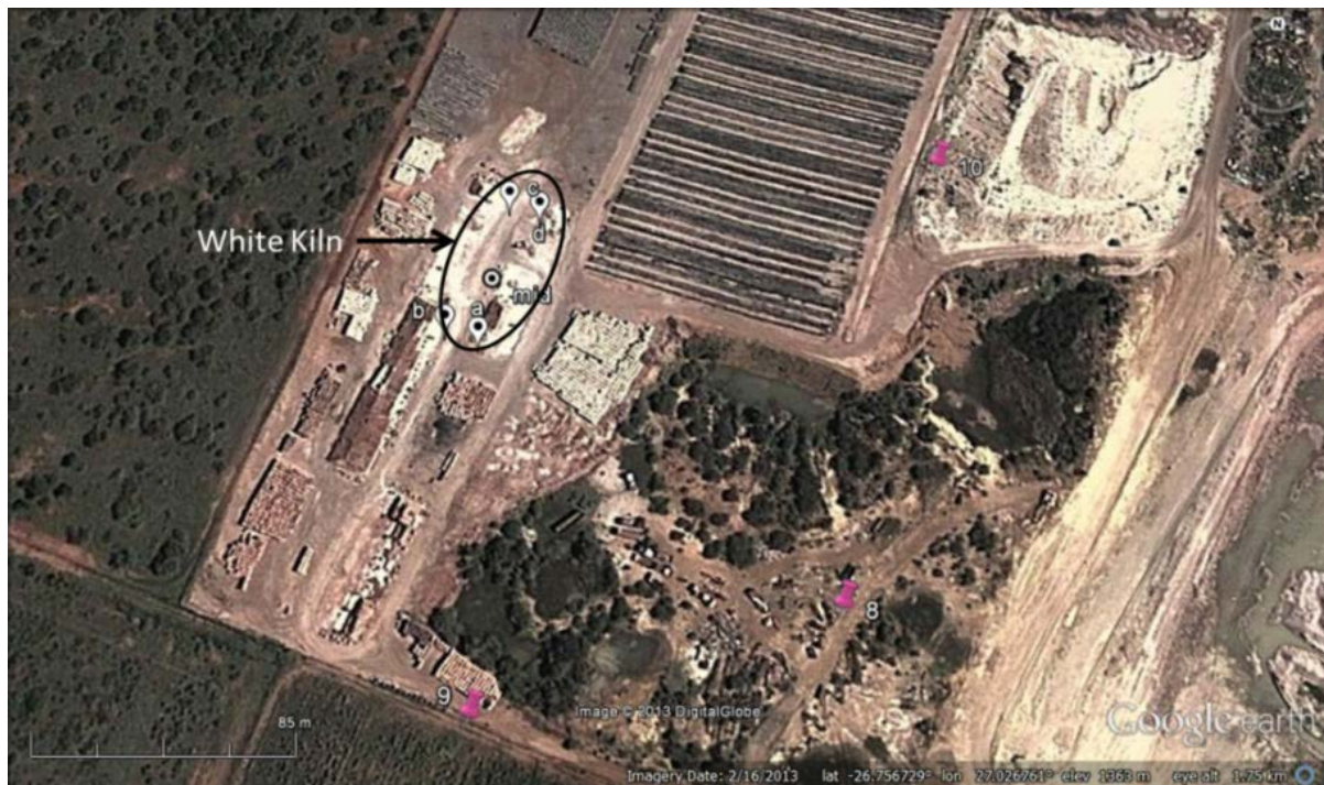
Figure 3-14: Location of samplers around white brick kiln at Berts Bricks, Potchefstroom
