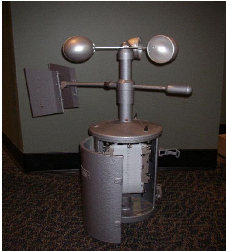
Figure 3-6: The Wilh. Lambrecht KG Gottingen® Cup Anemometer (Campbell Scientific, 2013)
