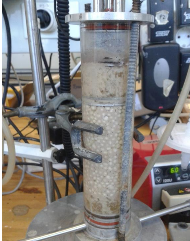
Figure 4.3: Reactor with mature biofilm during a steady state at D = 0.32 \text{ h}^{-1} ( S_o = 35 \text{ g.L}^{-1} )
