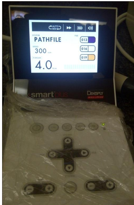
Figure 3.8: The X-Smart Plus Endodontic Motor (Dentsply/Maillefer) set at 300 rpm and 4 Ncm torque on display
