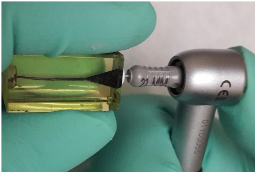
Figure 3.4: The M4 Safety reciprocating hand piece (SybronEndo) being attached to a size 0.8 stainless steel K-file (VDW)
