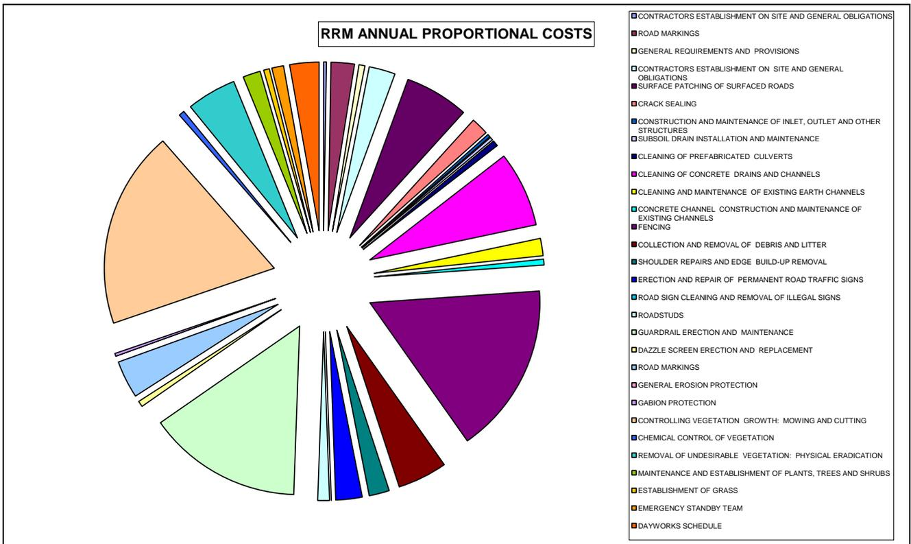
**Figure 2: Breakdown of routine road maintenance activities by cost (dual carriageway)**
