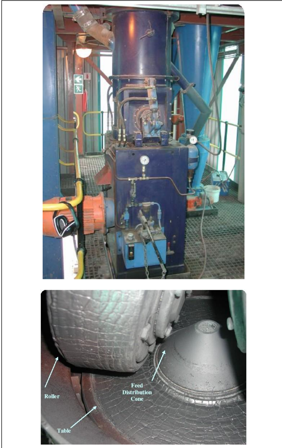
Figure 52: Views of the AARL Pilot Mill.
