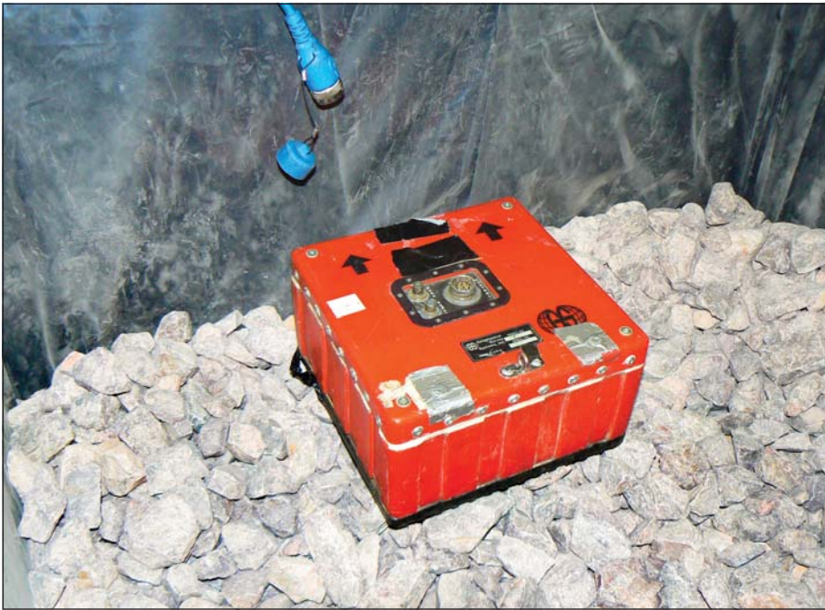
Figure 7 400 MHz antenna in the ballast box
