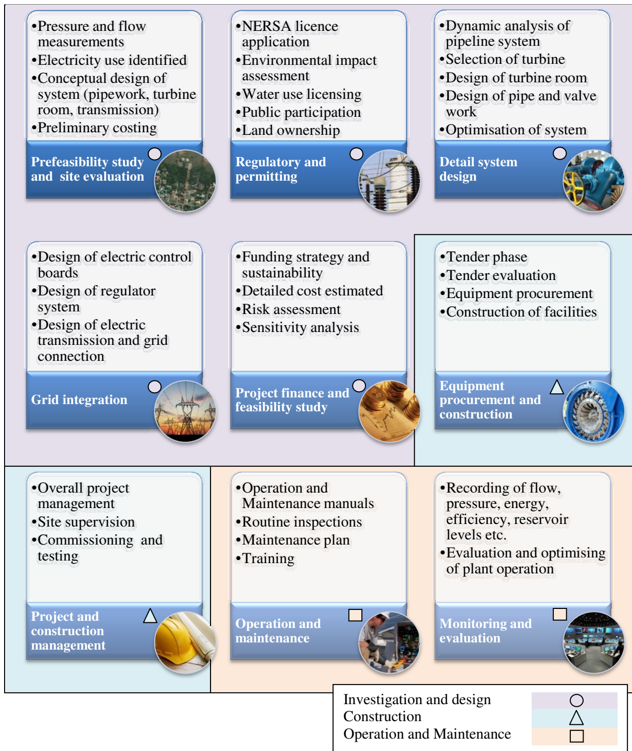
Figure 3-1: Conduit Hydropower Development Scope of Works
