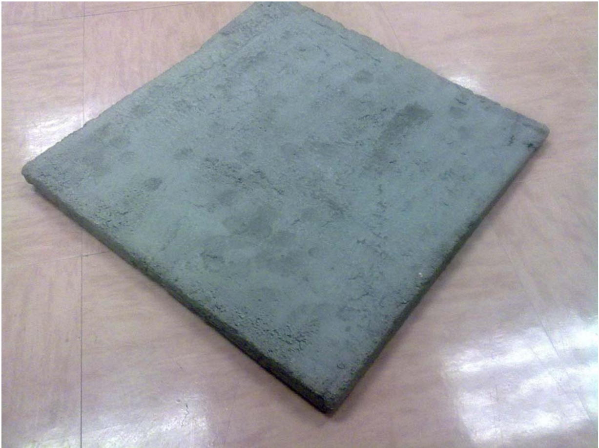
Figure 3.4: Example of a 25 x 300 x 300 mm composite plaster cement test sample
