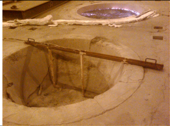
Figure 3.1-3: Empty mould with the prepared thermocouple rig positioned over it. The steel thermocouple holders were coated with a refractory to prevent reaction between the steel and the WCM
