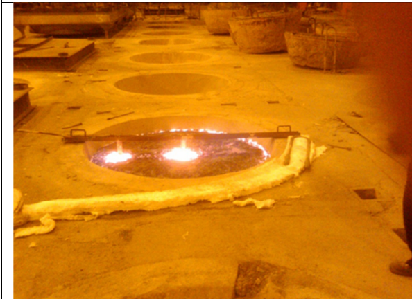
Figure 3.1-4: Molten WCM in a mould with the thermocouple rig positioned in the molten material. In the background of the picture (left) a typical lid positioned over a mould is visible.
