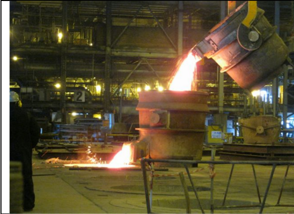
Figure 3.1-2: Casting of WCM from a 20t ladle via a bottom caster into the refractory lined mould
