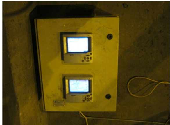
Figure 3.1-5: Two of the four channel digital recorders used for data collection
