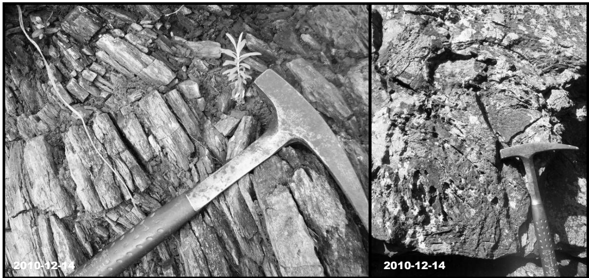
Figure 3.6: Siliceous schist (left) exposed at the northern ridge and basaltic pillow lava exposed on a plantation access road, both at Groenvally
