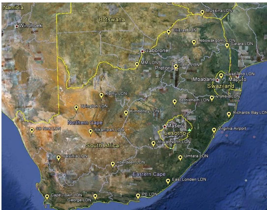
FIGURE 3.1 South African Weather Service (SAWS) Lightning Detection Network (LDN) sensor sites in 2012. Source: SAWS
