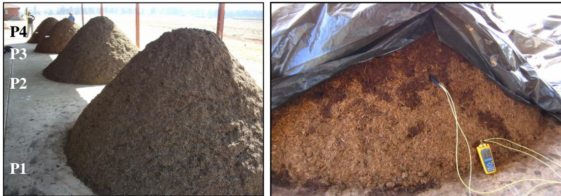
Figure 3.7 The 4 m 3 piles after initial mixing (left) and recording of pile temperature (right)
