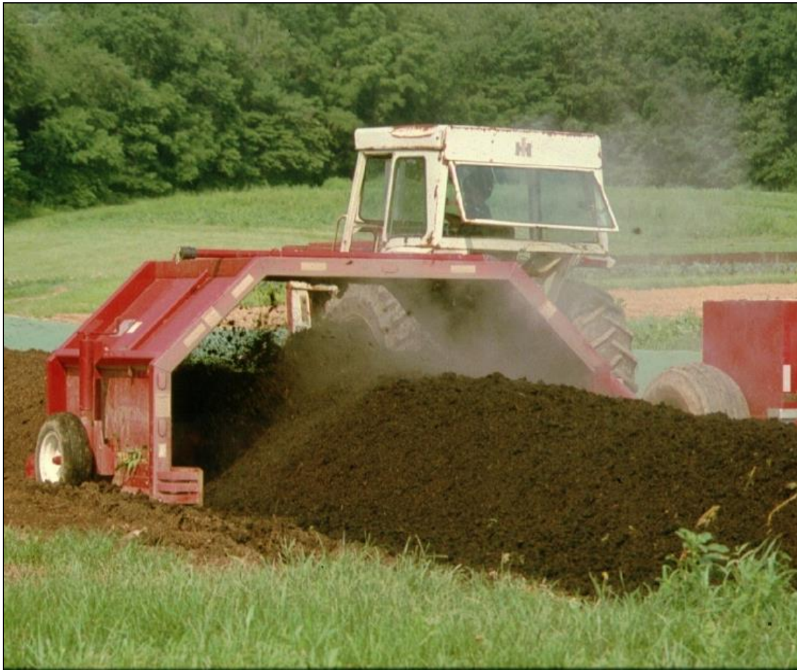
Figure 1.3 Feedstock of dining hall food scraps being composted in large-scale windrows that are mechanically turned/aerated (Brady and Weil, 1999)
