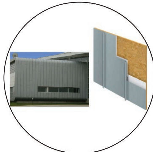
RHEINZINK Double Standing Seam with 500mm cover width, 0,8mm thick and single panel length of 5,00m used as vertical cladding fixed to steel sub frame.
