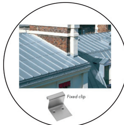
RHEINZINK Double Standing Seam with 500mm cover width, 0,8mm thick and single panel length of 5,00m with a roof pitch of 5° fixed to subroof with concealed RHEINZINK clips. Seams to be inside sealed with RHEINZINK sealing tape. Subroof to be 2400x1200mm x 80 mm thick layer of 35 Density yellow rigid polyurethane with a 9 mm thick Magnesium Oxide board laminated below and a 11 mm thick Oriented Strand Board (OSB) laminated on top. Sub roof fixed onto 100 x 50 20 m/s cold formed lip channel.
