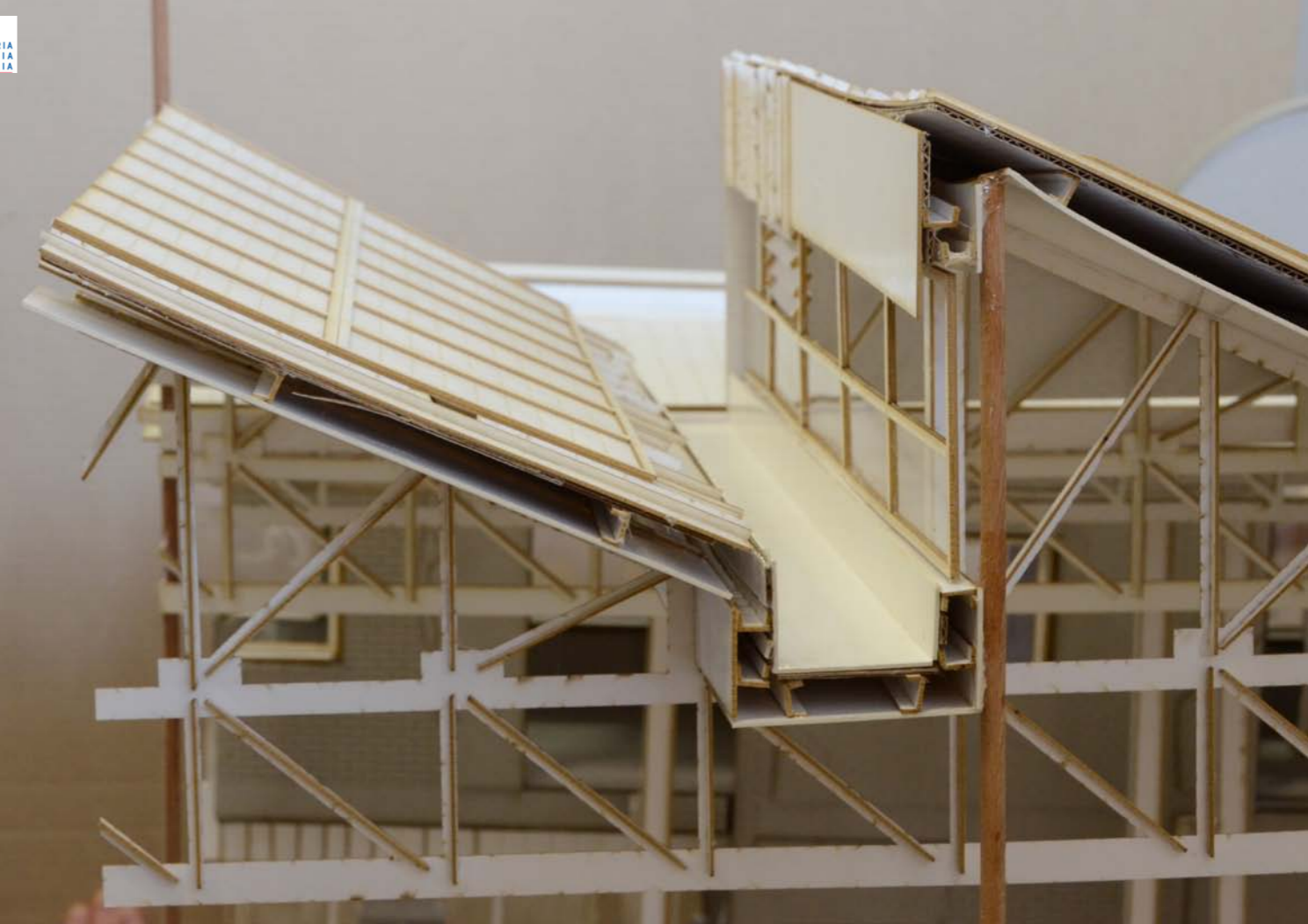
Figure 300: Model 2: sawtooth truss, box gutter and skylight detail (Author November 2013)
