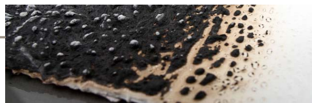
Figure 212: Burnt intumescent paint (Starkem 2011)
