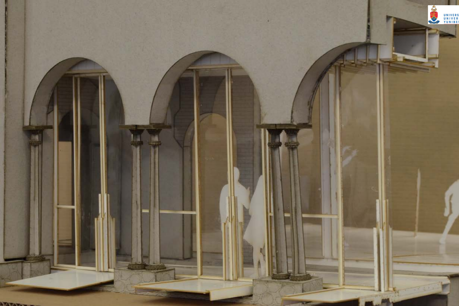
Figure 296: Model 2: new doors inserted into existing arches - wester facade (Author November 2013)
