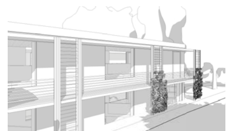
Figure 211 showing a draft computer perspective of the lighter steel structure of the office facade (Author 2012)
