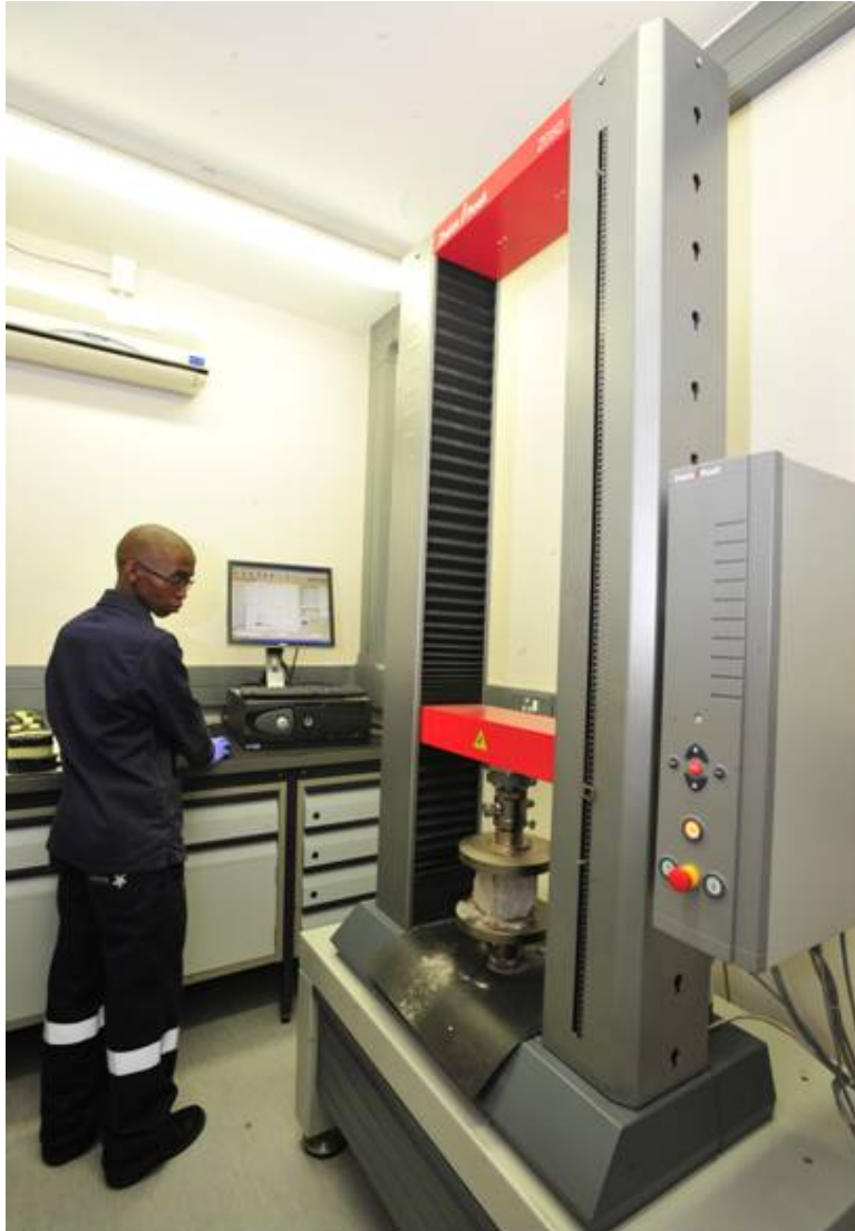
Figure 3.13 Picture of UCS determination in a Z050 Zwick Roell compression machine
