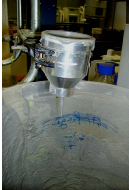
Figure 3.6b Blockage in a modified flow cone
