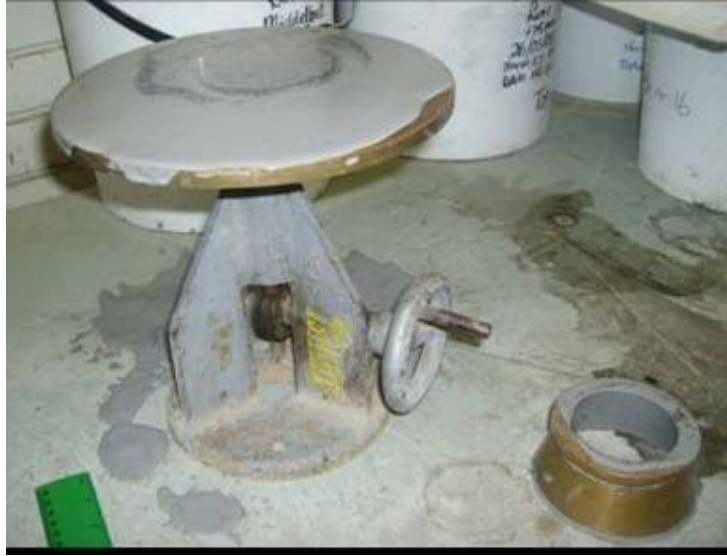
Figure 3.3b Illustration of paste overflowing the table top
