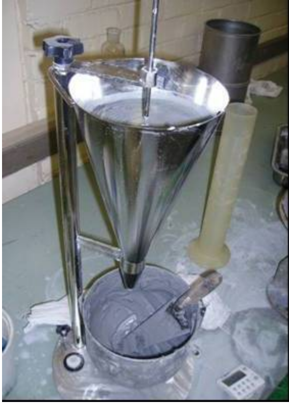
Figure 3.6a Blockage in a standard flow cone
