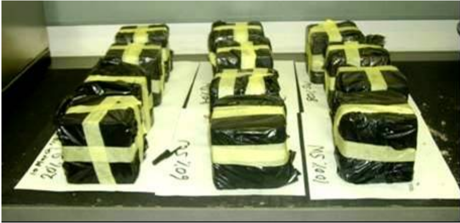
Figure 3.12 Curing of paste samples under controlled conditions
