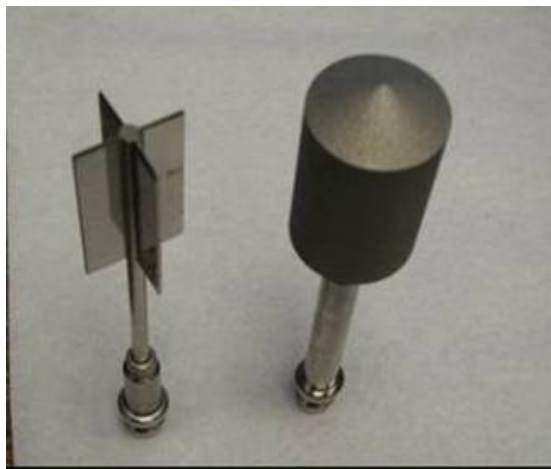
Figure 3.10 Photo of vane and bob systems
