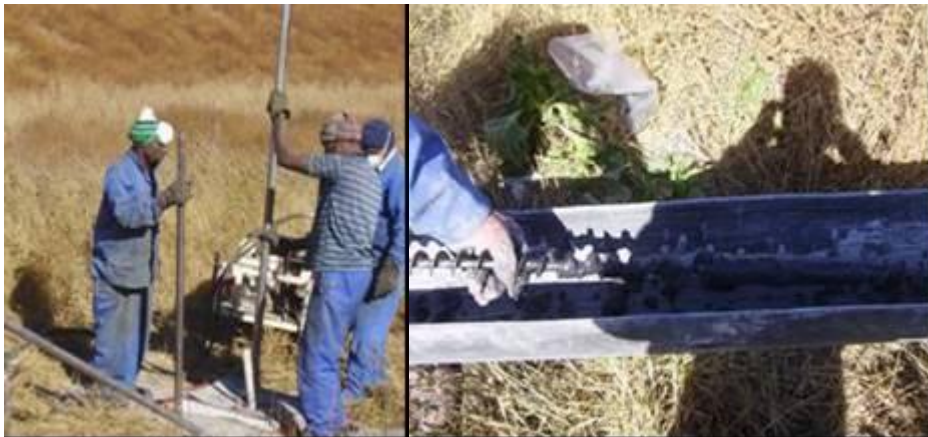
Figure 4.6 Illustration of sampling in a FAD using Auger drill
