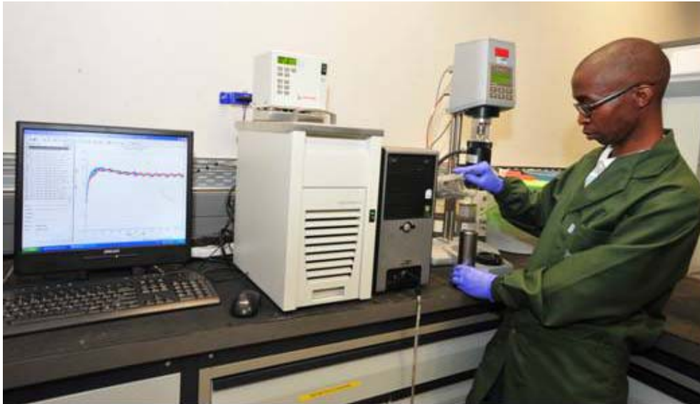
Figure 3.7 Photo of a modern vane rheometer in use
