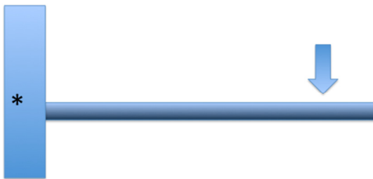
Figure 6-3: Schematic illustrating a cantilever bending test. The specimen is fixed to the one end (asterisk) and a load at the opposite end.
