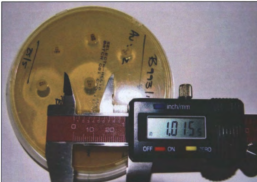
Figure 20 Measurement of the halo around each antibiotic containing disc tested, using a digital vernier calliper. According to the halo's size, bacteria were classified as sensitive, intermediate or resistant to that particular antibiotic.
