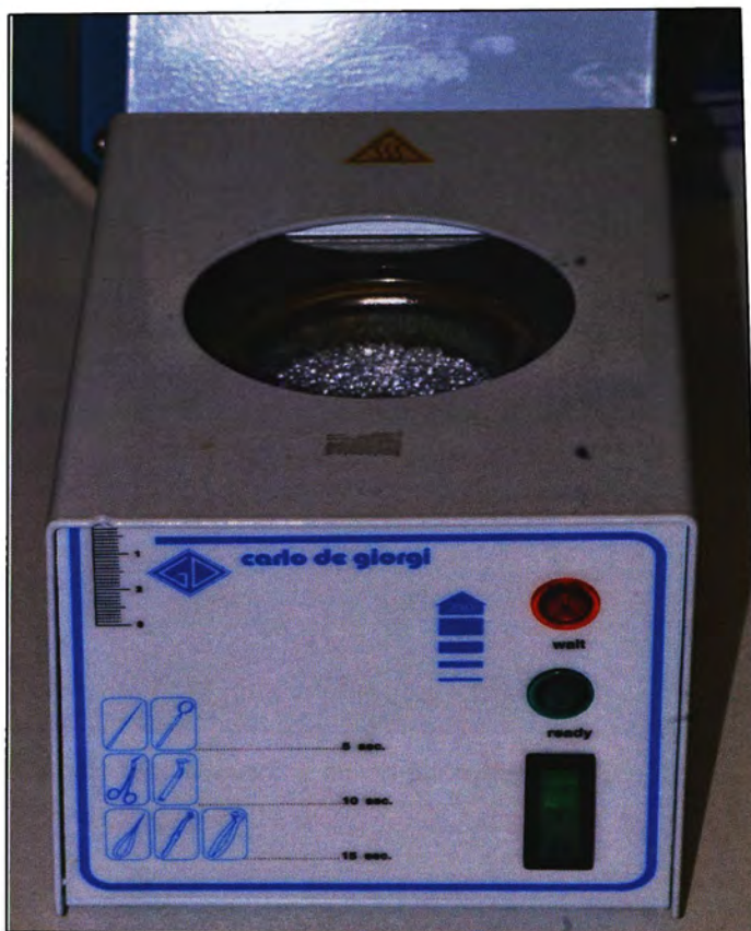
Figure 12 All the instruments inserted into the RC were sterilised in a bead steriliser before they were employed in the sampling process to avoid any contamination of the samples.
