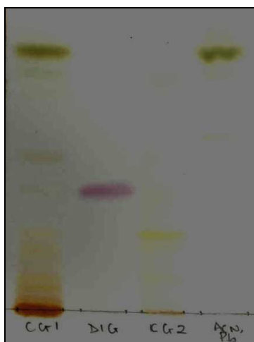
Figure 7-3: Chromatogram of extracts sprayed with Kedde reagent. Lanes from left to right: CG1 (cardenolides), digitoxin, CG2 (cardiac glycosides) and Pb-washed acetone extract (one wash) developed in EMW solvent system.
