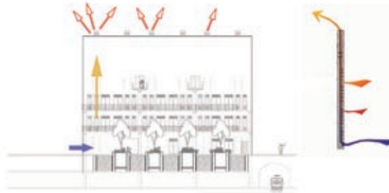
FIG. 9.3.4.1.7 Elevation and section right of ATRIUM well as a measuring element to absorb thermal energy and act as a ventilator
