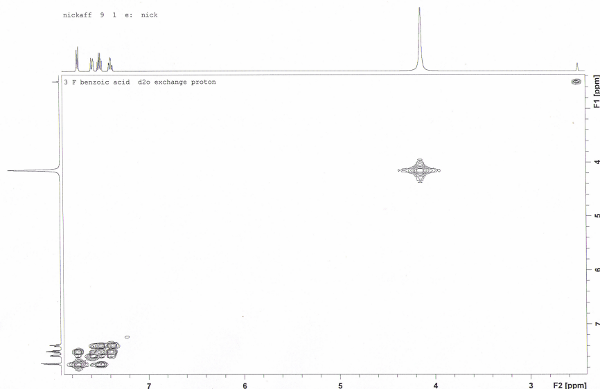
Fig. 5.12 COSY NMR of 3-fluorobenzoic acid
