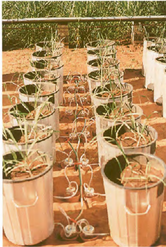
Plate 3. Each pot was independently linked to a vacuum trap.
