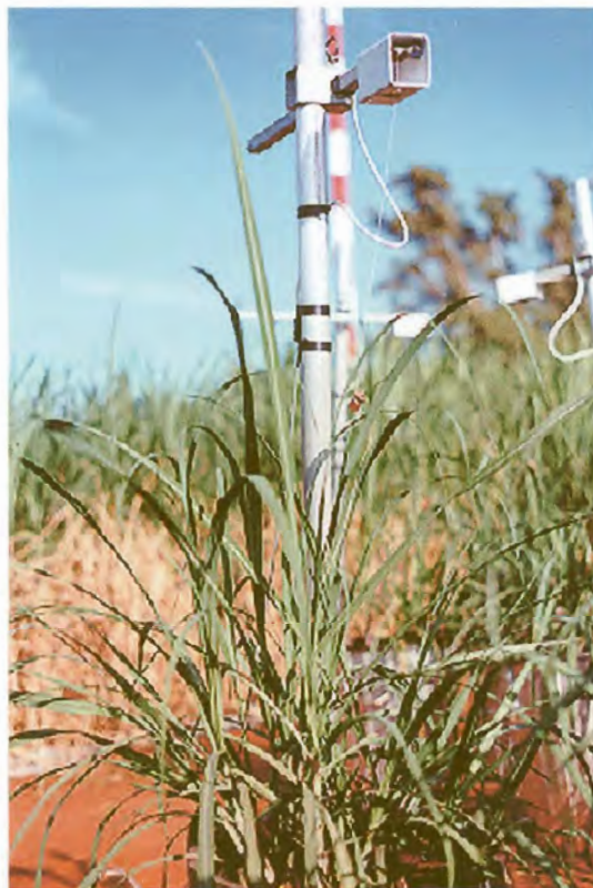
Plate 4. Growth transducers were used to measure plant extension rate.
