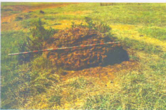
FIG. E.11 - Ferricrete block consisting of iron concretions.
