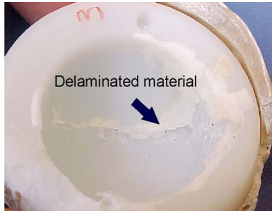
Figure 5.2: A cup with delamination
