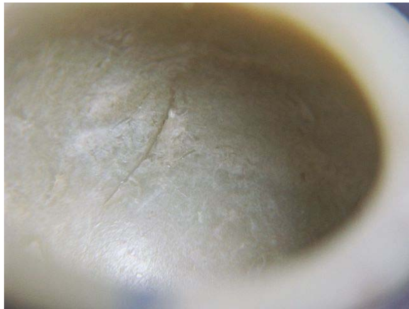
Figure 6.8: Acetabular cup with severe scratches on inside
