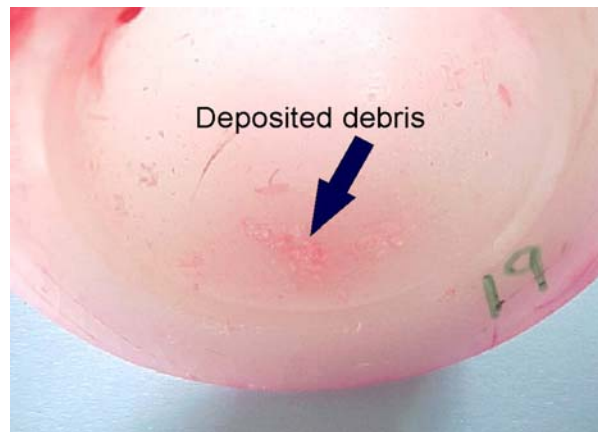
Figure 5.4: Deposited debris – coloured with liquid dye penetrant to make it more visible
