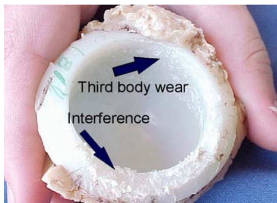
Figure 5.8: A cup with evidence of interference and subsequent damage
