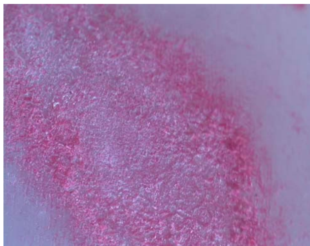
Figure 6.24: Area with adhesion wear (magnification x 40)
