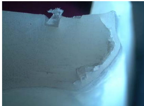
Figure 5.22: Magnification (x 10) of defect on rim of cup
