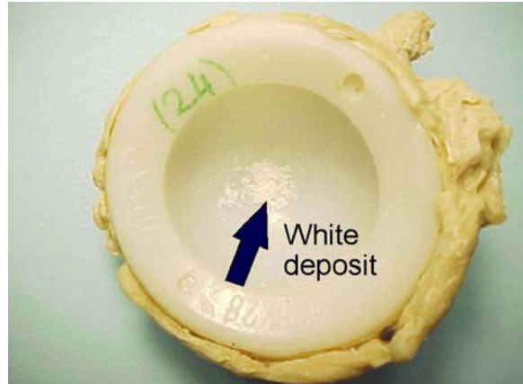
Figure 5.12: White deposits on inside of cup and brown discolouring
