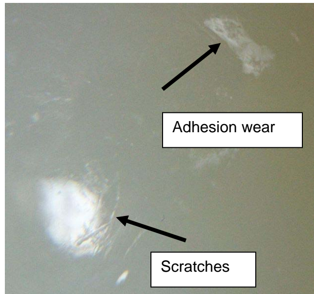
Figure 6.10: Bearing area with signs of large scratches and area with adhesion wear
