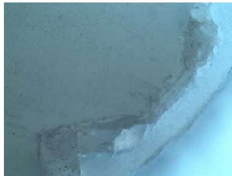
Figure 5.23: Magnification (x 20) of defect on rim of cup
