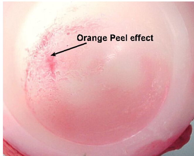
Figure 4.5: Cup treated with dye penetrant showing “orange peel” effect indicating plastic flow of material
