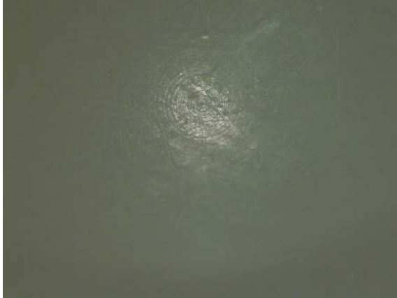
Figure 5.35: Machining marks visible in acetabular cup
