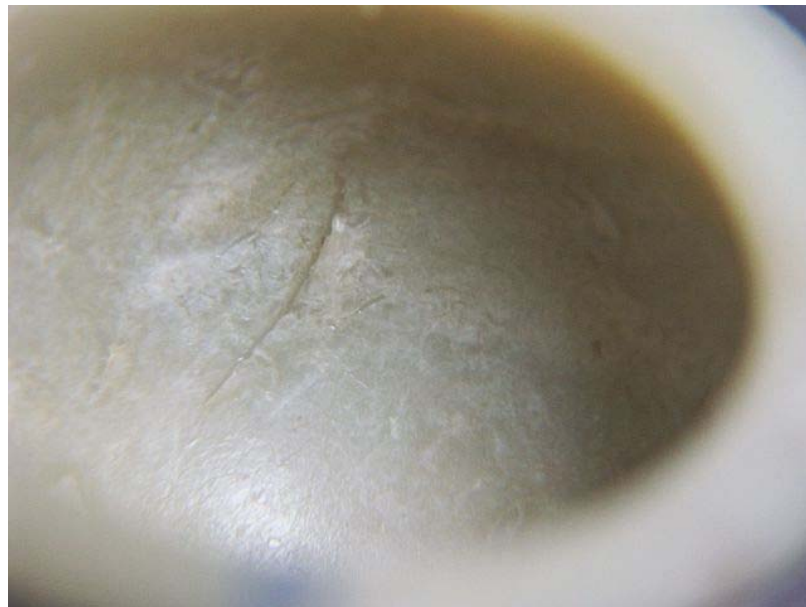
Figure 6.8: Acetabular cup with severe scratches on inside
