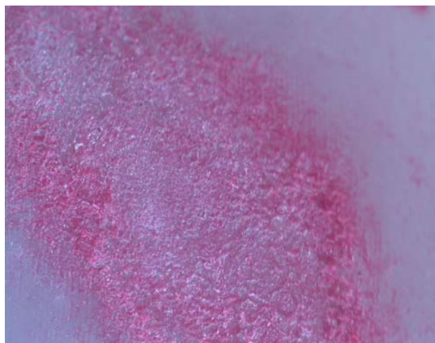
Figure 6.24: Area with adhesion wear (magnification x 40)
