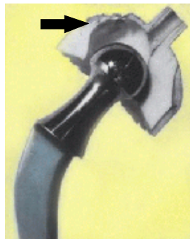
Figure 1.2: The early prosthesis as designed by Sir John Charnley. Note the migration of the femoral head into the Teflon.
