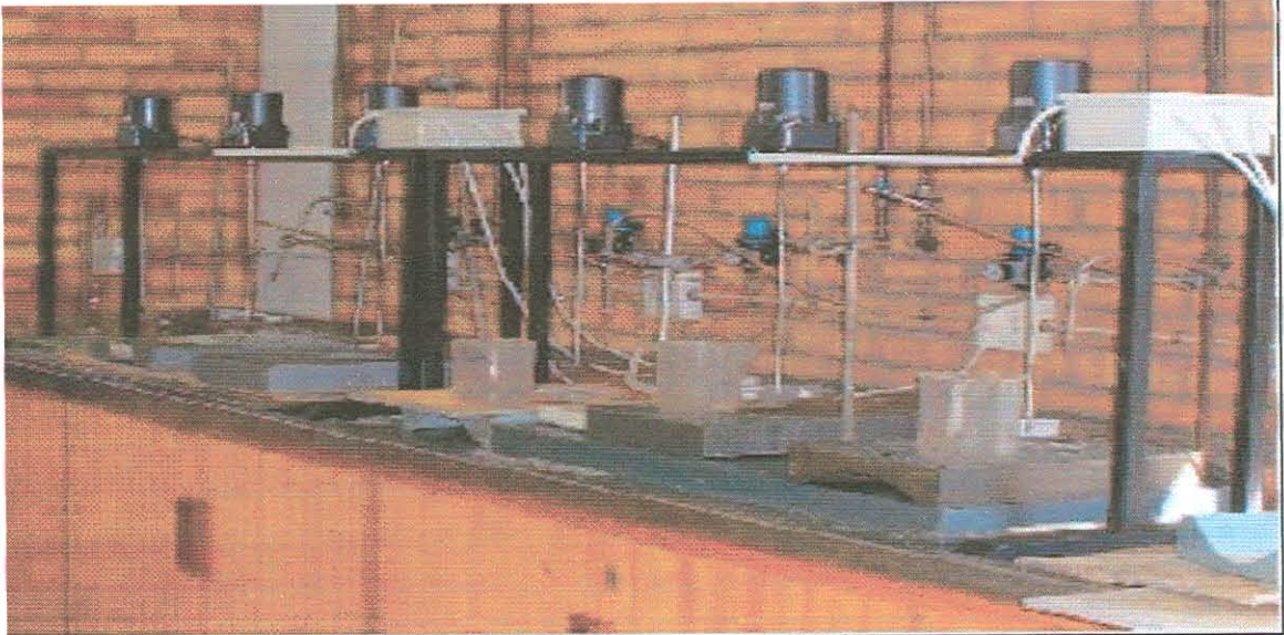
Plate 2: Batch test conducted in 1L beaker reactors
