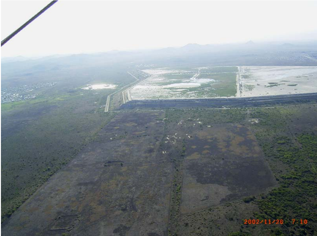
Figure 4.9: An example of an area source (tailings dam) (North West Ecoforum, 2002).
