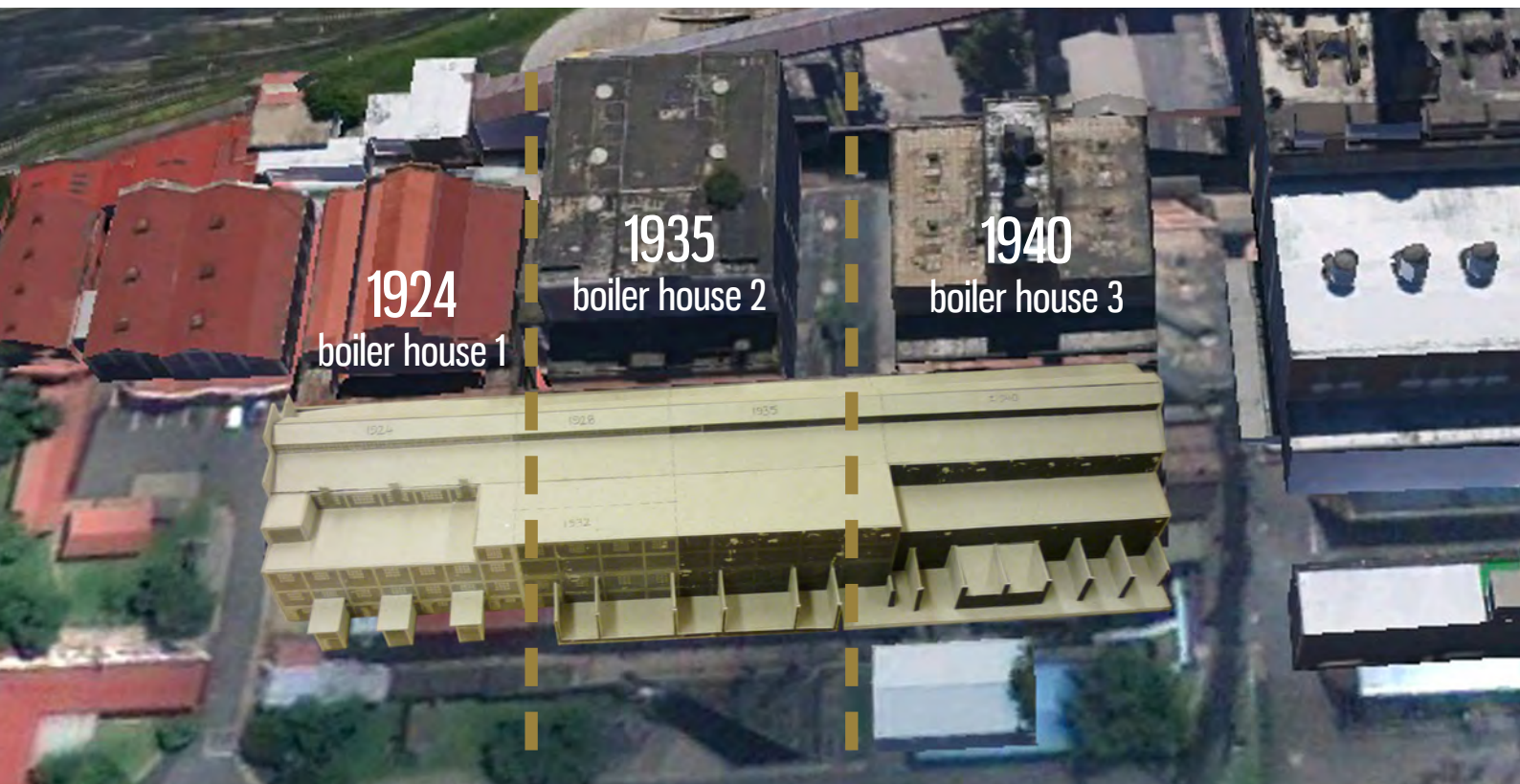
[Fig. 125] Showing the three main phases of progressive construction of the old Turbine Hall
