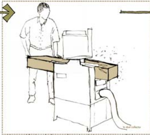
Manageable size planks are shaped and planed to correct thicknesses with a thickness planer, only a small amount of material is removed.
