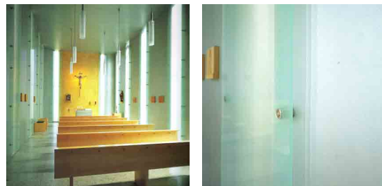
Fig. 7.35 and 7.36 Tirschenreuth Chapel, Germany, Bruckner & Bruckner. Illumination of the interior through a series of vertical cuts in the wall
