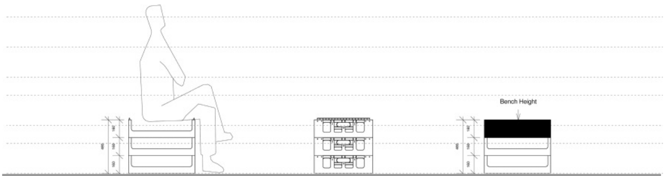
Figure 156. Developing bench height from crate height
