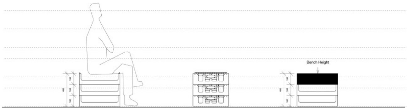
Figure 156. Developing bench height from crate height
