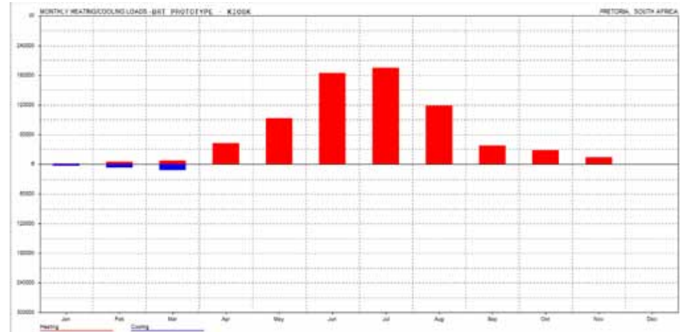
Graph 13-03: BRT station - Heating and cooling required for Kiosk station [Source: Author].
