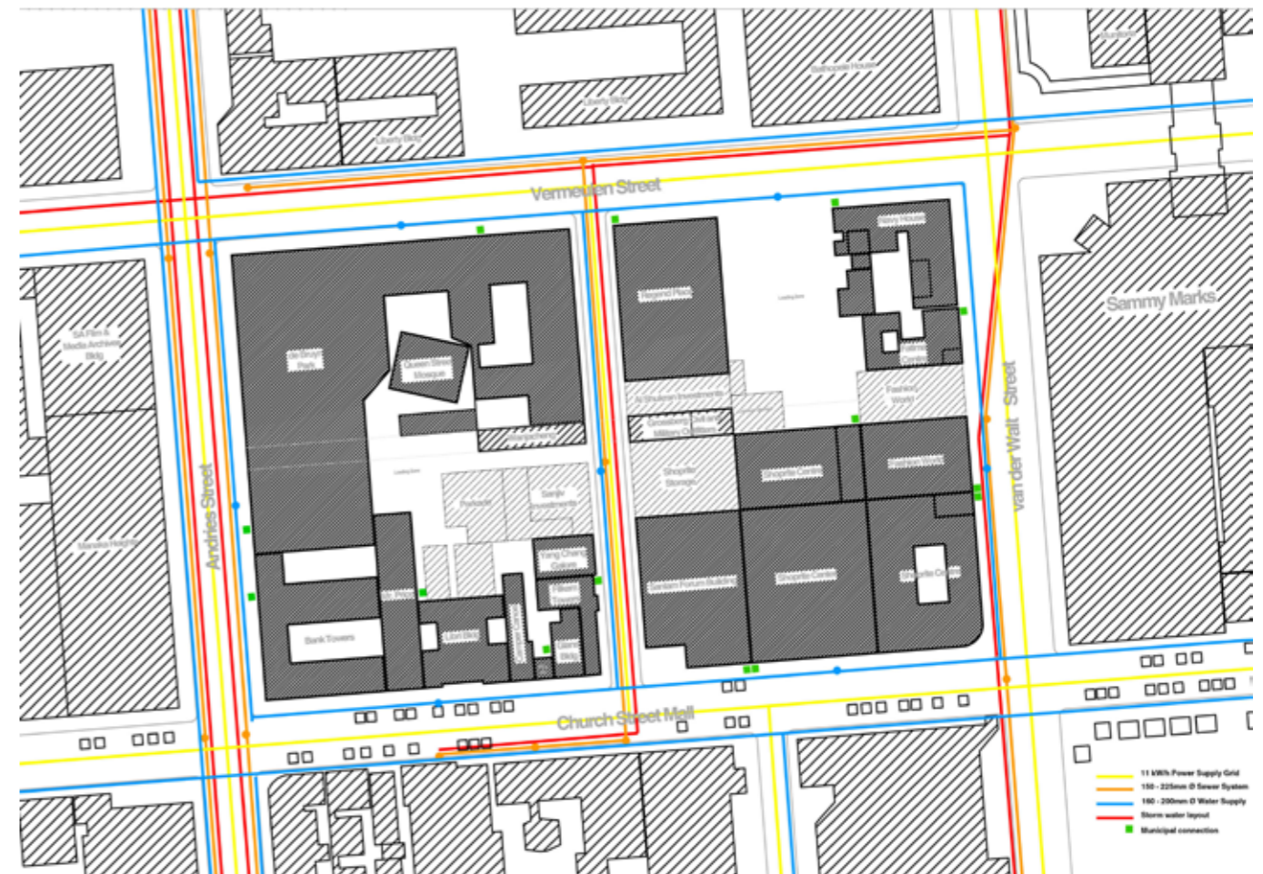
[Figure 9_3.] Existing municipal infrastructure around and on site.
