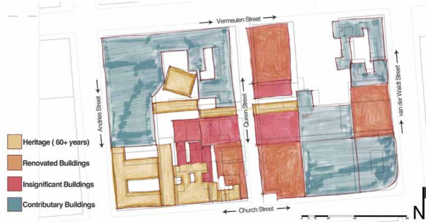
[Figure 3_17.] Significance. Illustrates where the weaknesses lie concerning contributory fabric. The block core has deteriorated because it has no street frontage and thus development didn't take place here.
