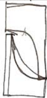
Figure 263. Two 38x114mm pieces of timber are cut to 600mm lengths. The ends are rounded and a slot is cut in each end for a casters to fit through. The two pieces are fixed together with a shiplap joint and secured with wood-glue and wood-screws .A caster is placed in each slot and fixed to the wood with wood-screws. Matching holes are cut in the base of the drum to accommodate the casters. The assembly is placed in the bottom of the drum (Author,2010).
