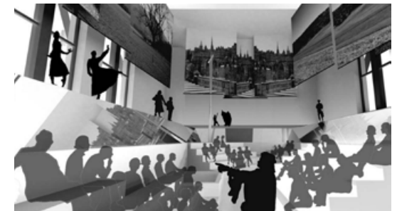
Figure 28. Interior based on Edouard Autant's plan and section. Actors play improvised scenes in lower area between audience bleachers and choreographed drama on upper surrounding stage. Tilted mirrors reflect action behind spectators (Read, 2006).
