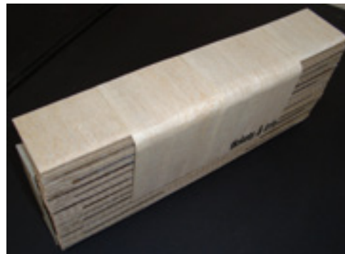
Figure 196. 1:1 Prototype of cardboard tube building blocks (Author, 2010)
