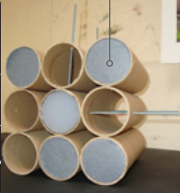
Figure 196. 1:1 Prototype of cardboard tube building blocks (Author, 2010)
