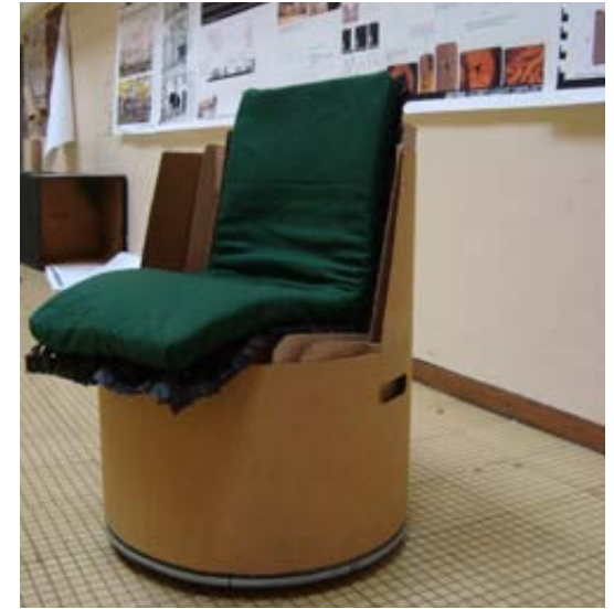
Figure 267. 1:1 Prototype of cardboard swivel chair with upholstered covering (Author, 2010)
