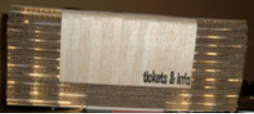
Figure 200. Model illustrating lighting effect of layers of open cell X-board & acrylic sheet lit from behind with a CFL (Author, 2010).
