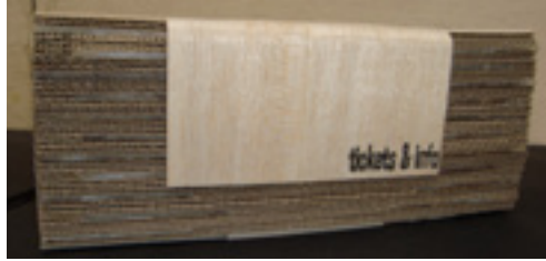
Figure 200. Model illustrating lighting effect of layers of open cell X-board & acrylic sheet lit from behind with a CFL (Author, 2010).
