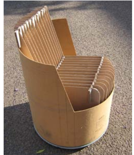
Figure 265. Sheets of cardboard was cut according to the chair profile and stacked next to each other inside the chair to create a seating surface. A 450 x 1000 mm rubber mat is woven from 40mm wide strips of the inner tube of a vehicle tyre. A 400 x 950 x 40 mm piece of foam is covered with a felt cover that can be removed and washed. The covered foam is attached to the rubber mat by pressed-it clips. The 'pillow' is then placed onto the seating surface of the chair to increase comfort & acoustic absorption. The pillow itself can also be used as temporary movable seating with the rubber mat as durable substrate providing a non-slip grip (Author,2010).
