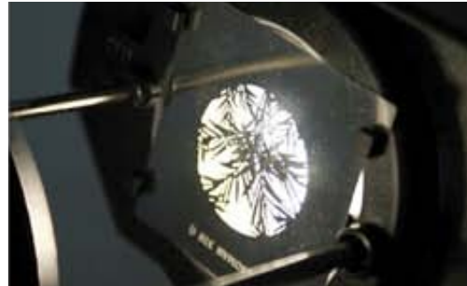
Figure 217. Gobo inserted in the focal plane of a luminaire (GoboMan, 2010).
