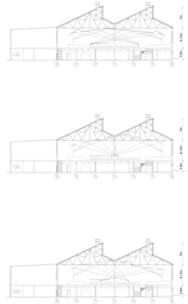
Figure 242. Determining the reflection angles of the acoustic panels (Author,2010)
