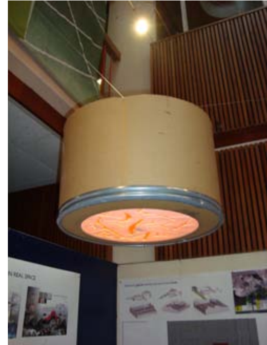
Figure 222. 1:1 Prototype of cardboard drum diffuser (Author, 2010)
