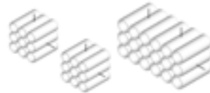
270x270x270 mm Building blocs constructed from nine pieces of 75ø cardboard tubes, cut to size and fixed together with clear silicon in 270x270x270 cubes. Cubes are fixed to each other with 4ø threaded rod through corresponding pre-drilled holes.
