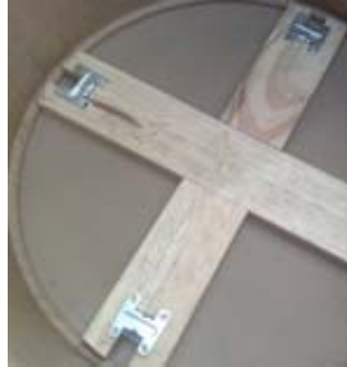
Figure 263. Two 38x114mm pieces of timber are cut to 600mm lengths. The ends are rounded and a slot is cut in each end for a casters to fit through. The two pieces are fixed together with a shiplap joint and secured with wood-glue and wood-screws .A caster is placed in each slot and fixed to the wood with wood-screws. Matching holes are cut in the base of the drum to accommodate the casters. The assembly is placed in the bottom of the drum (Author,2010).
